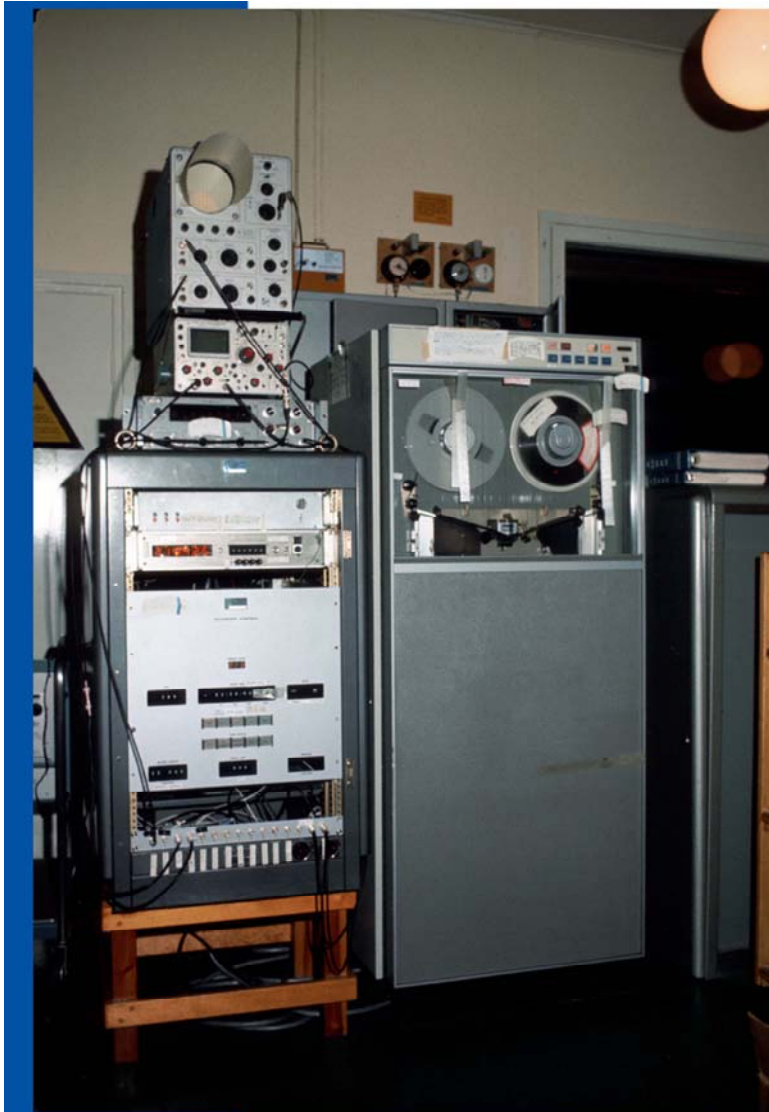
Mark I VLBI data recording system.
