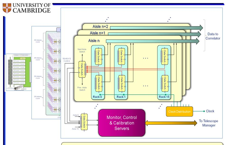
256 racks in 16 aisles Flexible beamforming High speed switched network Overlayed monit. & control
