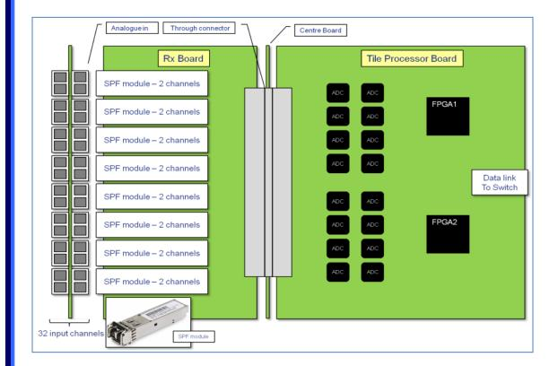
Analogue inputs 16 dual pol. antennas Digitise and beamform
