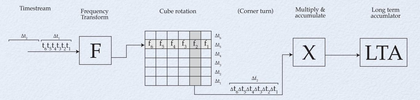
Must reorder data so X operation can accumulate successive products & keep bandwidth to the LTA sane.
