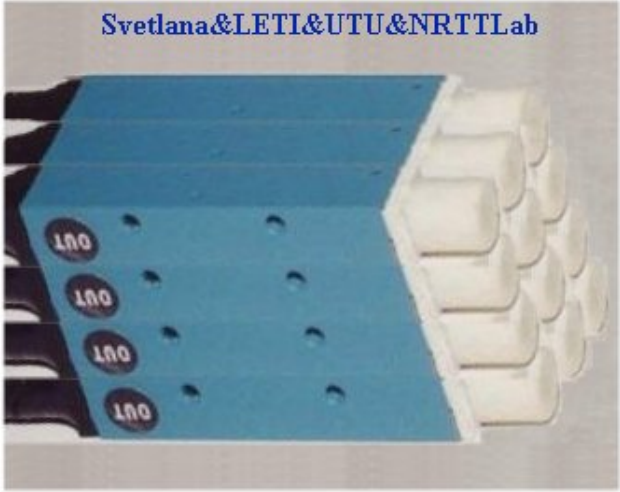
3x8 beam passive FPA prototype at 10 mm and one FPA element BP in the array
