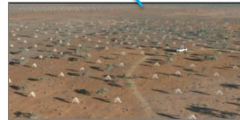
SKA2_LOW Low Frequency Aperture Array Stations 3 million antennas
