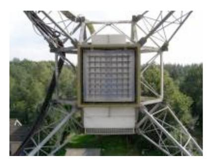
Telescope:  $12 \times 25$  m Beam-size: 15 arcsec Fov: 8 deg<sup>2</sup> (FPA) Bandwidth: 300 MHz Frequency range: 900 -- 1700 MHz (z < 0.85) line sensitivity (150 kms<sup>-1</sup>): 0.15 mJy/beam (12 hr) (1 $\sigma$ ) 0.52 mJy/beam (1 hr)
