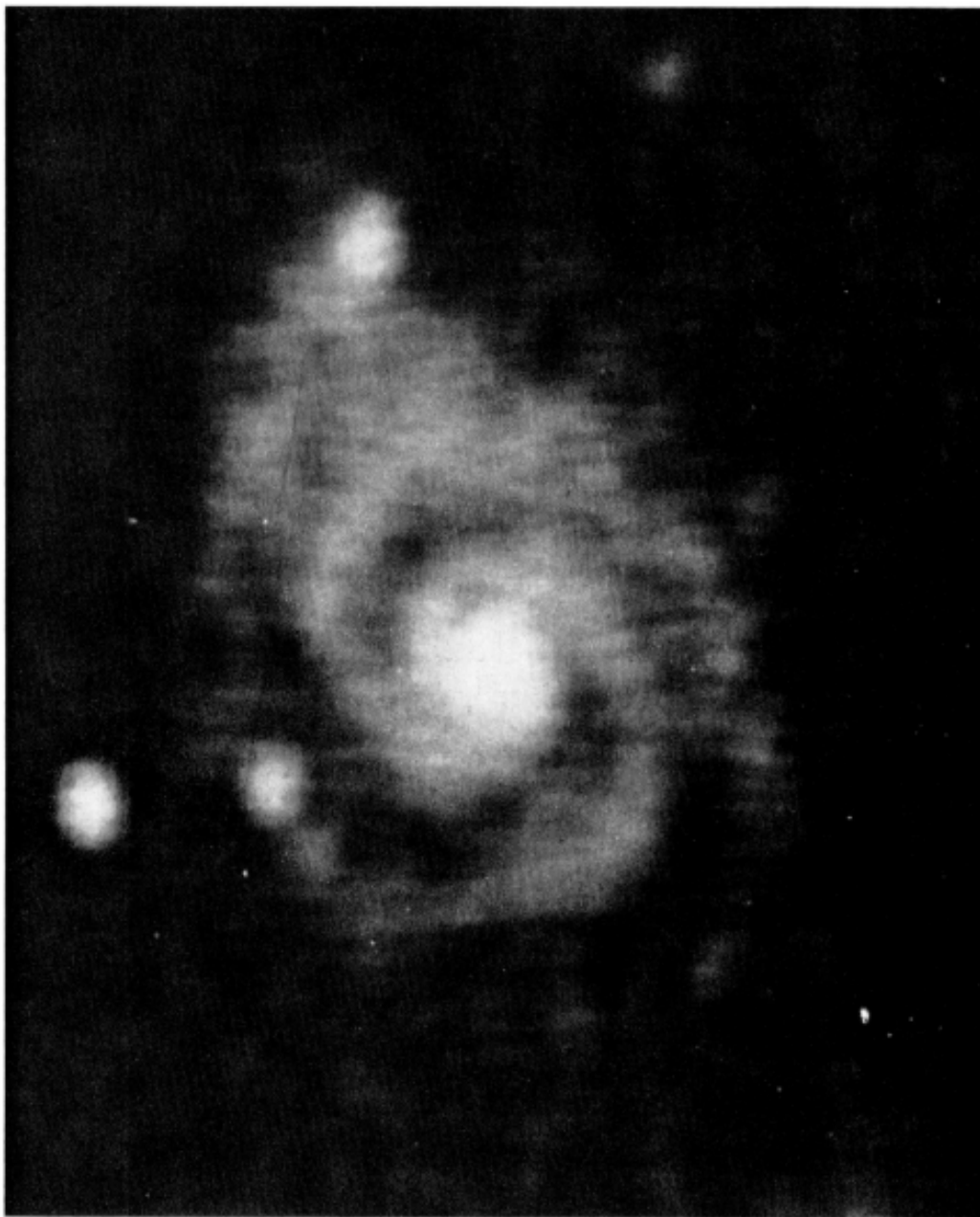
Fig. 2 Radio picture of M51 and NGC 5195 made by Jaffe using a computer-controlled cathode-ray tube with camera attached. Extra noise is added to the radio picture due to 50 Hz interference in the positioning of the beam of the cathode-ray tube
