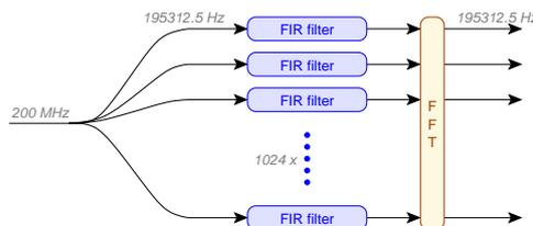
Figure 2: The first-stage PPF performs a 1024-point FFT over the output over 1024 FIR filters.
