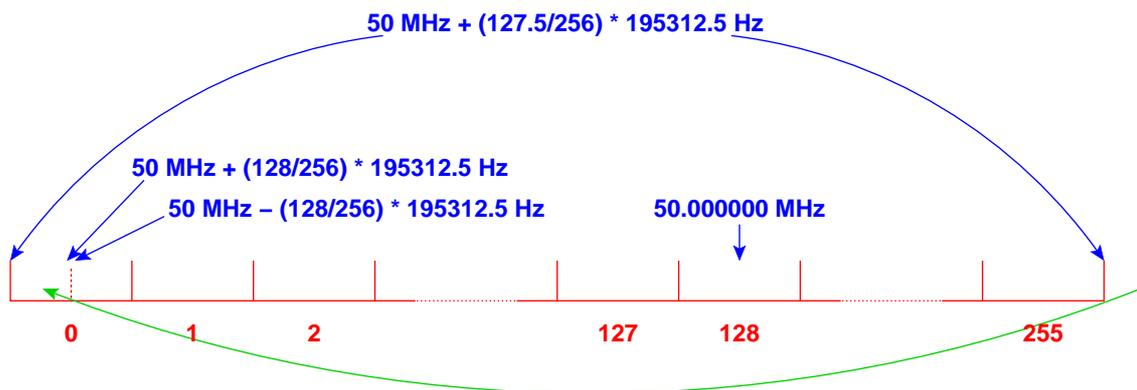
Figure 6: The PPF shifts the frequency by half a channel. The red numbers below indicate the channel numbers.
