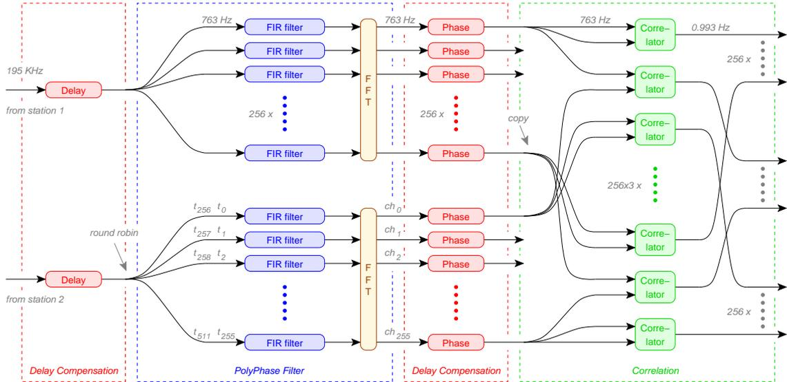
Figure 4: Signal processing on CEP for one subband.
