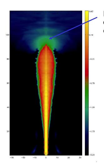
External material displaced in front of the jet
