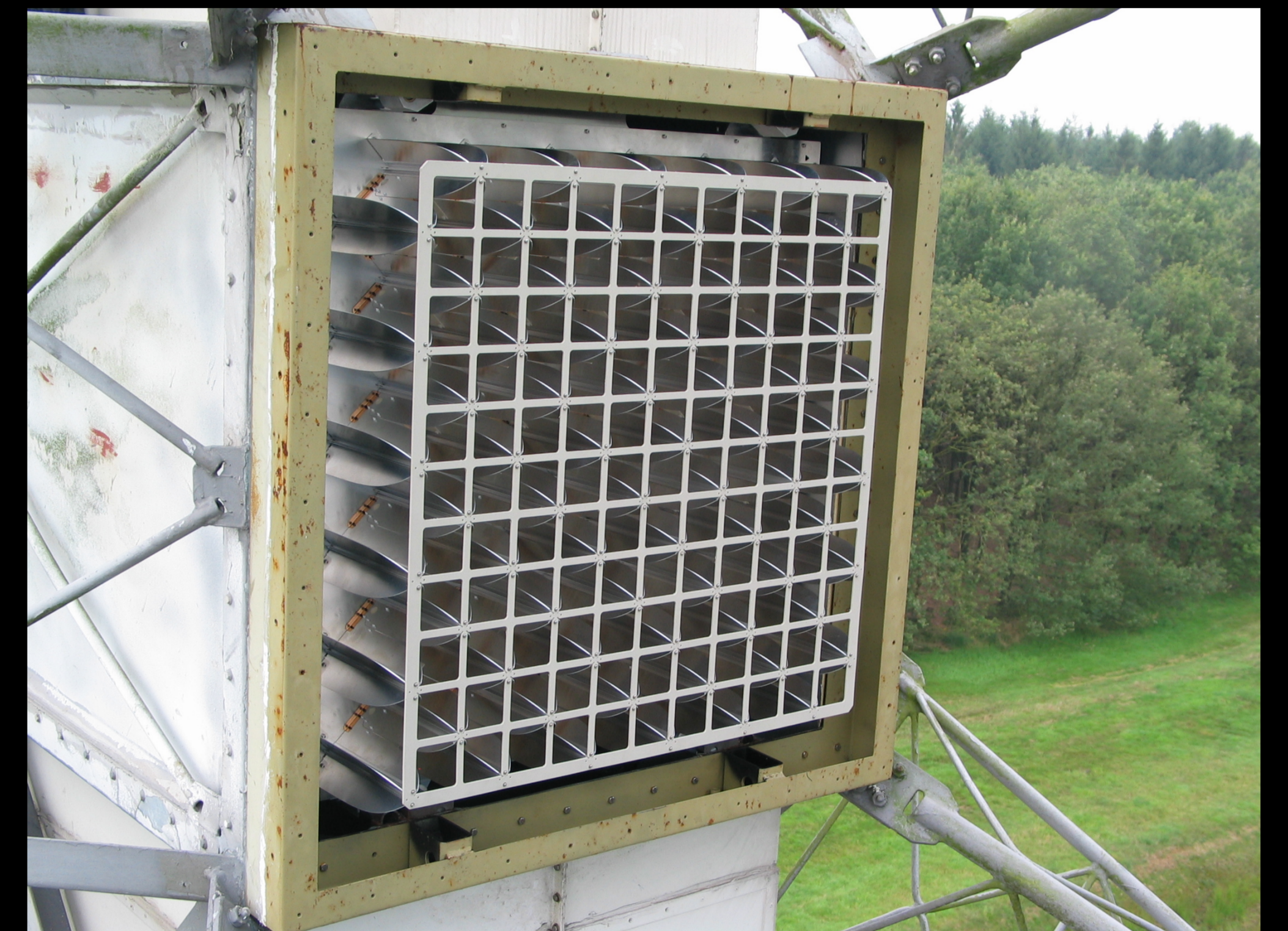
Left: detail of an Apertif receiver system. It consists of 121 separate small antennas. The current WSRT corresponds to only a single such antenna. Each WSRT dish will be equipped with such an array of 121 antennas. Right: a full Apertif receiver mounted in the focal plane of one of the WSRT dishes.
