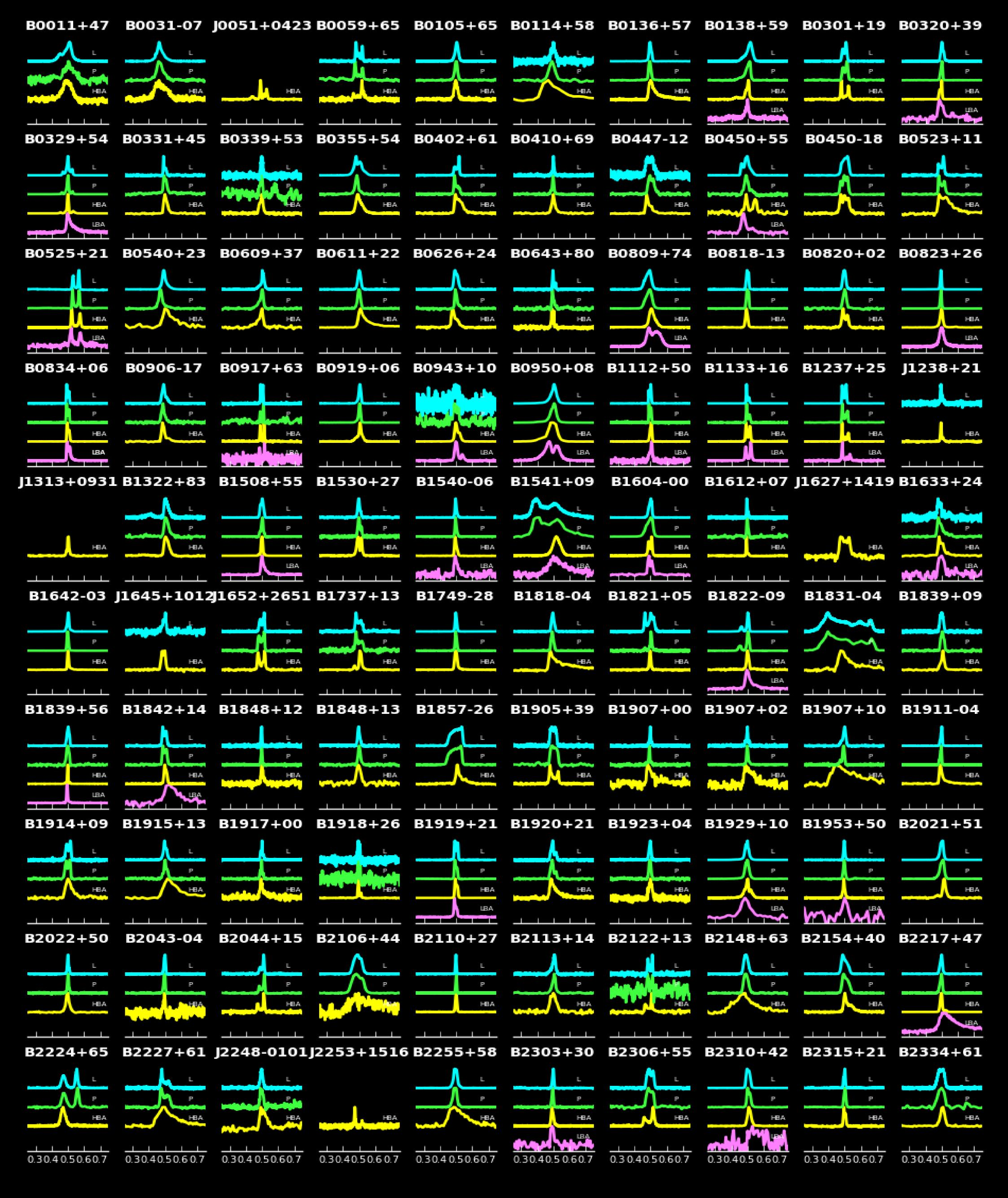
LOFAR'S FIRST 100 PULSARS: Observations of 100 pulsars with LOFAR LBAs (40 Mhz) and HBAs (140 MHz), WSRT (at P-band, 400 MHz) and the Lovell Telescope (at L-band, 1400 MHz). The evolution of the pulse profile with frequency help us explore the properties of the magnetosphere of the pulsar and of the medium between us and the pulsars.
