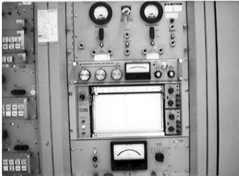
Old Square-law detector and chart recorder system as used by NASA (DSN)
