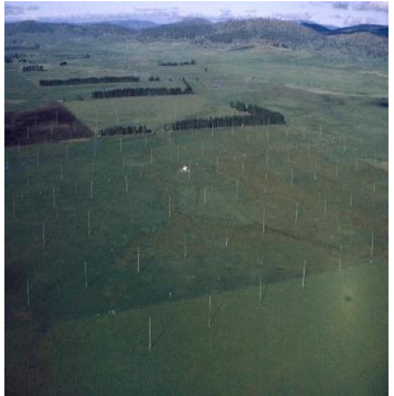
Reber's 2MHz Square km dipole array.
