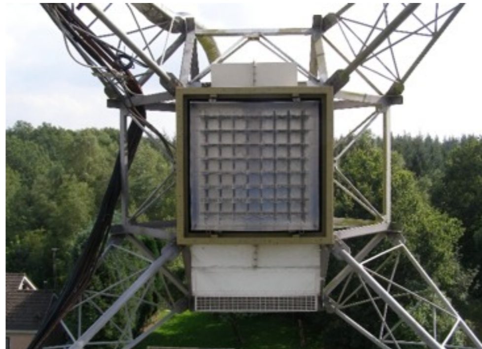
A focal plane array demonstration system (Digestif) installed on one of the telescopes at WSRT. (ASTRON)
