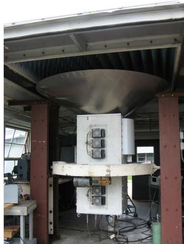
Roof closed with ambient absorber for hot load.
