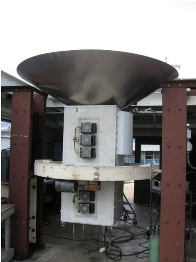
Array exposed to sky for cold load.
