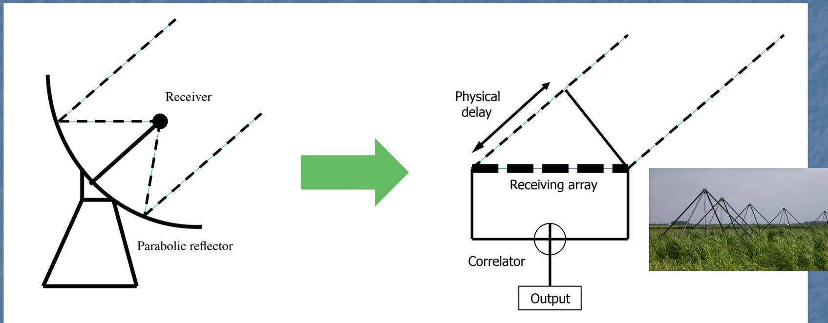
Enormous flexibility: **electronic beamforming** and ‘software telescope’
