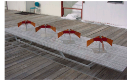
Prototype of the High Frequency Antenna (developed at Haystack Observatory) which will operate between 110 and 220 MHz. The final design will probably consist of a 4x4 array of these kind of antenna's together with an RF beamformer.
