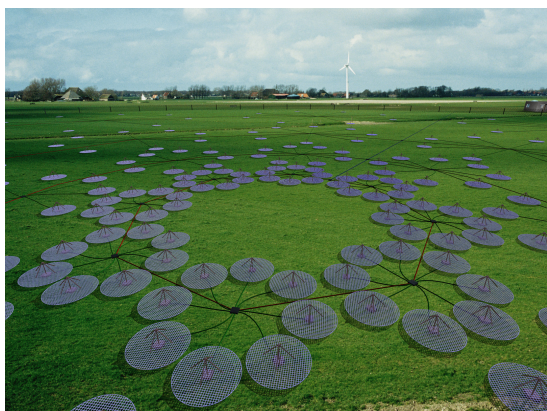
The figure above gives an artist's impression of one of approximately 100 LOFAR stations. The antennas in the station form a phased array, producing one or many station beams on the sky. Multi-beaming is a major advantage of the phased array concept. It is not only used to increase observational efficiency by allowing the telescope to point to different regions of sky at the same time, but may also be vital for calibration purposes. Effectively each station beam is a collection of many monochromatic beams centred at the same position on the sky.
