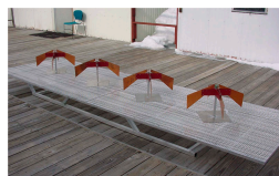
Prototype of the High Frequency Antenna (developed at Haystack Observatory) which will operate between 110 and 220 MHz. The final design is shown.
