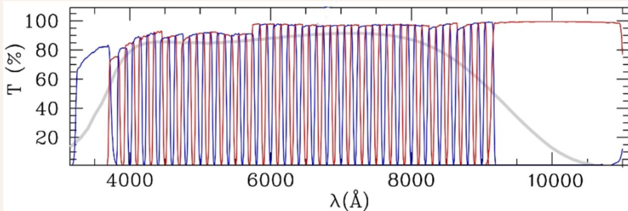
**54 narrow-band** ( $\sim 130\text{\AA}$ ) + **2 medium-band filters** + *ugr*
