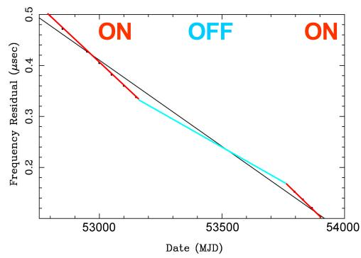
Increase in slow-down rate during 'ON' state  $(dv/dt)_{ON}/(dv/dt)_{OFF} = 1.8 \pm 0.1$
