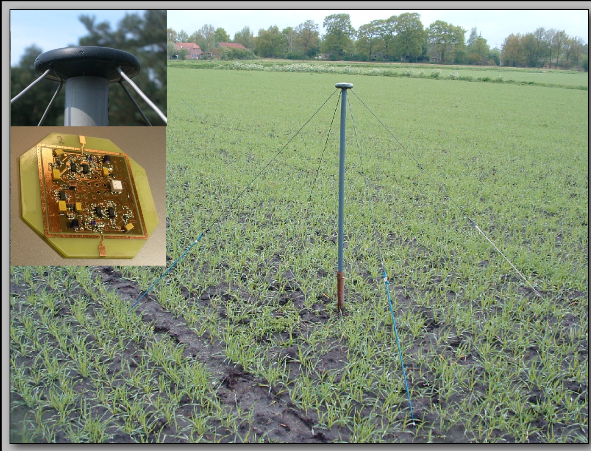
Low band antenna: 30 – 80 MHz 48/96 antennas per station
