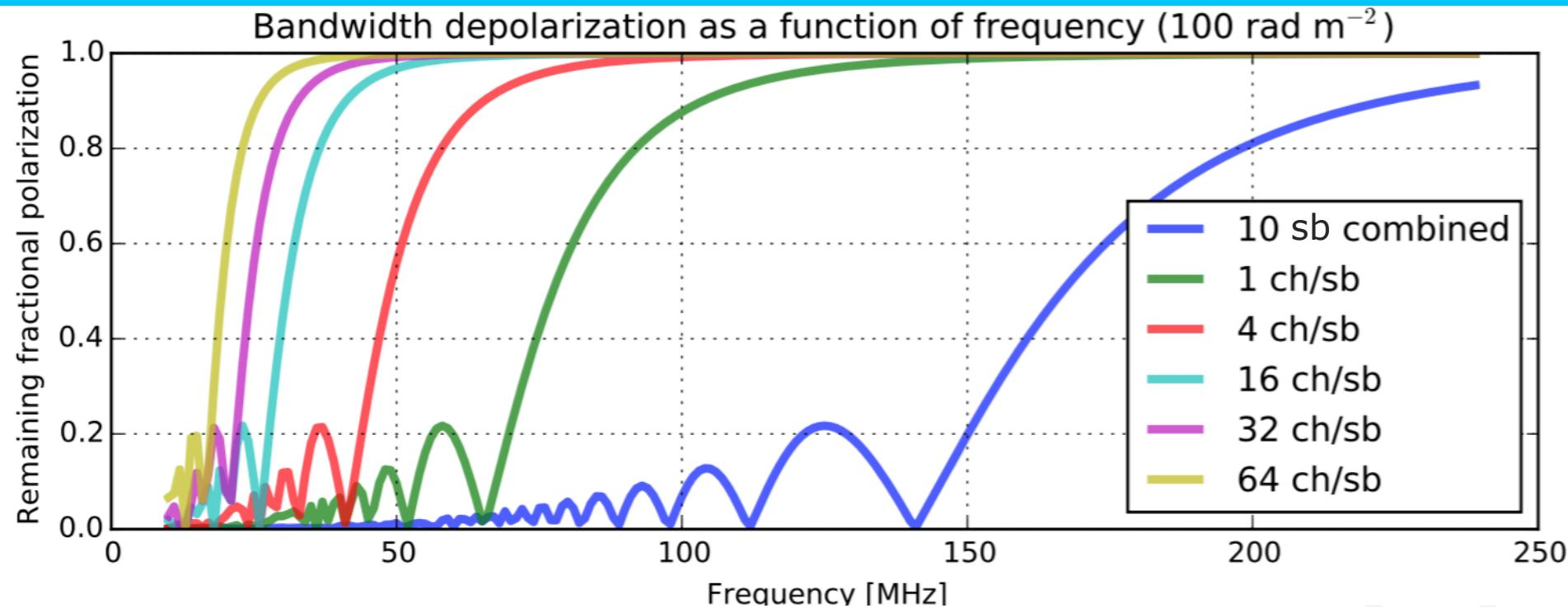
When frequency averaging your LOFAR data the signal can completely depolarize. Carefully choose averaging factors for LBA and HBA polarimetry!
