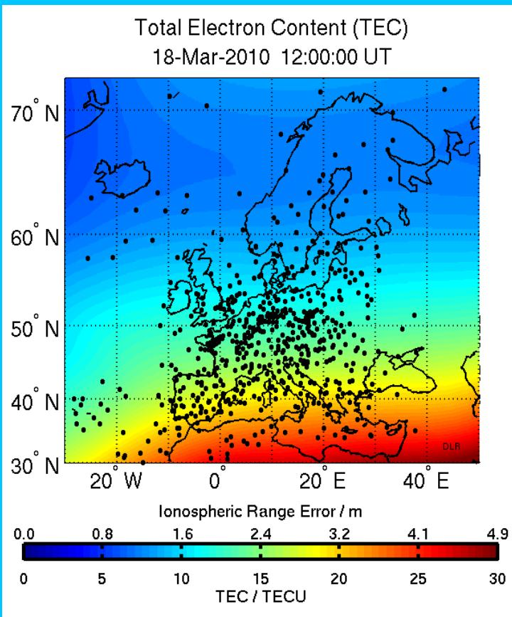
Stations apart >10 km see different ionosphere, i.e. different amounts of ionospheric Faraday rotation.
