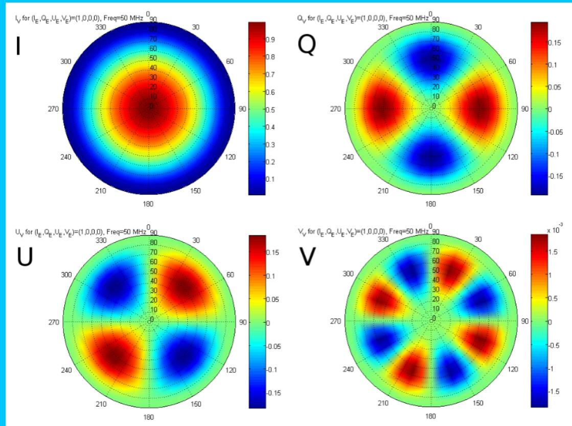
Calibrating the polarization response towards the pointing center is enough to obtain low leakage wide field maps
