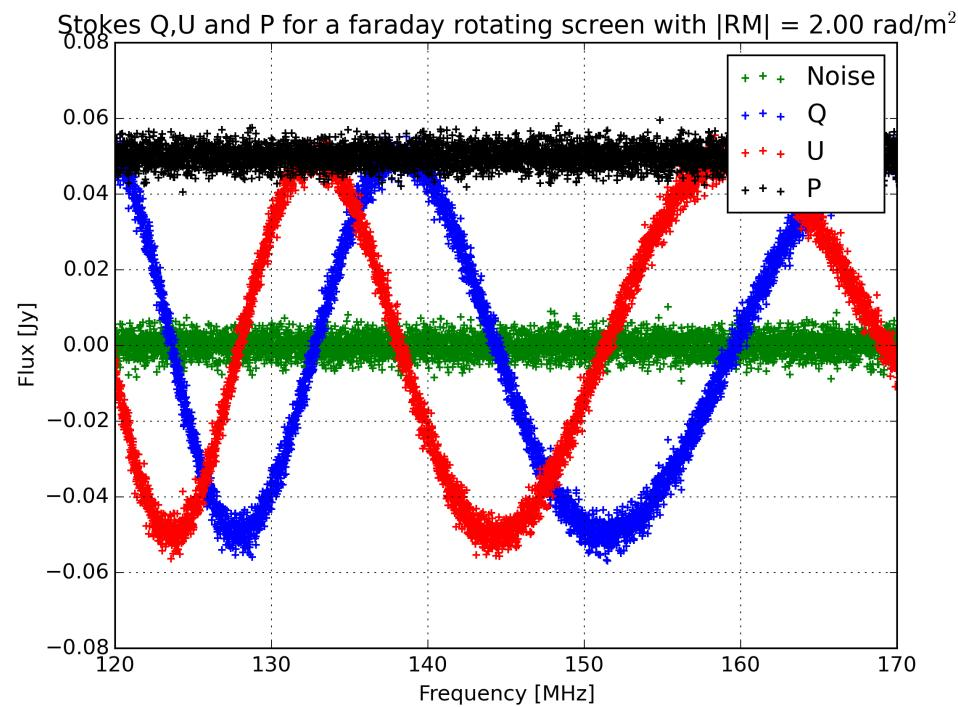
When frequency averaging your LOFAR data the signal can completely depolarize. Carefully choose averaging factors for LBA and HBA polarimetry!
