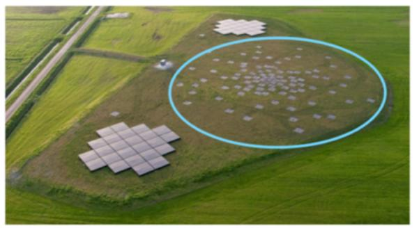
Frequency: 30-75 MHz (8 x 2 MHz bands) Resolution: ≤100 arcsec Sensitivity: ≤15 mJy/beam Area: 20,000 square degrees Number of Fields: 660 Simultaneous ~10° beams: 5 Test observations resuming
