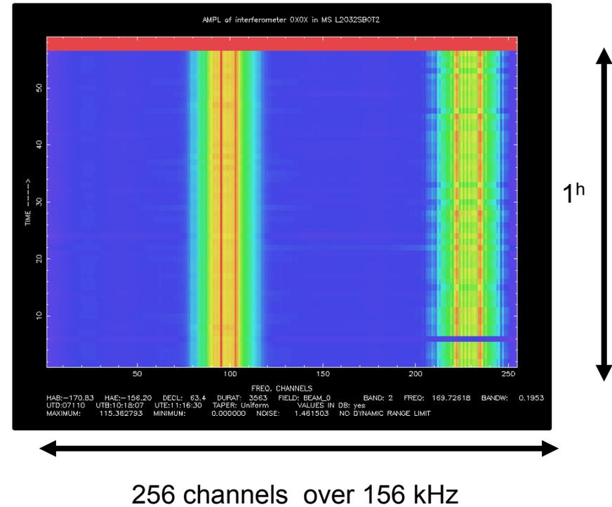
100 - 200 MHz spectrum of a LOFAR HBA dipole (at 195 kHz resolution) (Dec 2007)
