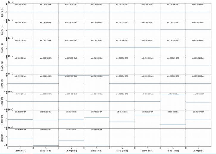
**4th** iteration of calibration after correcting for **PA** + **bandpass** + **beam** + **FR**
