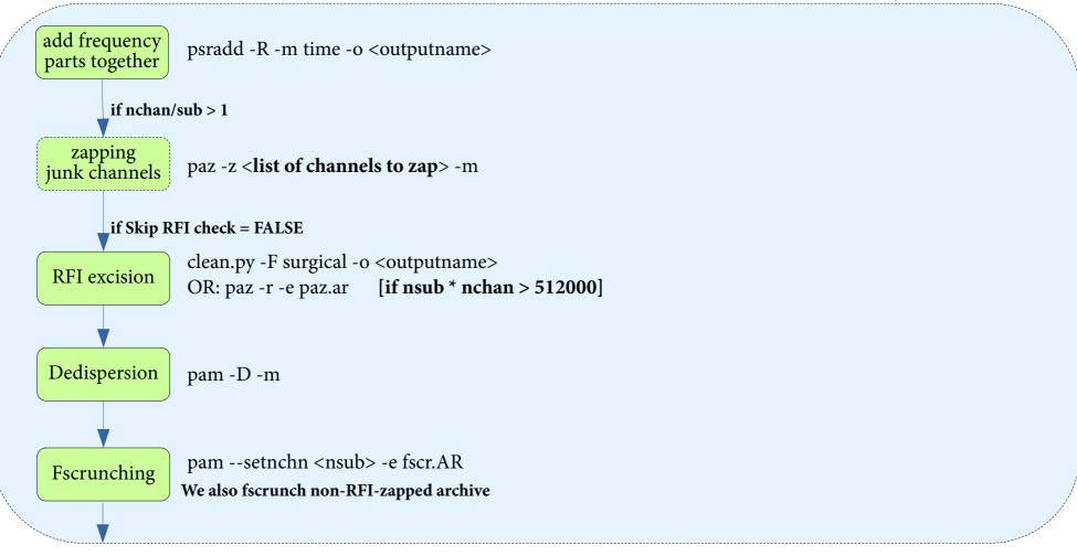
If there are 16 chan/sub, we need to zap every 16th channel, then list becomes «0 15 31 47...» This is necessary, as when 2nd PPF is used, the first channel in each subband gets corrupted
