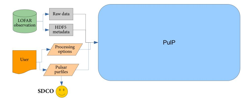
**Parfiles**: if parfiles are not given toPulP, then based on the target name it will try to find the corresponding pulsar in the ATNF catalog. If no pulsar is found in the catalog, PulP will look for the brightest pulsar in a given SAP and fold it.
