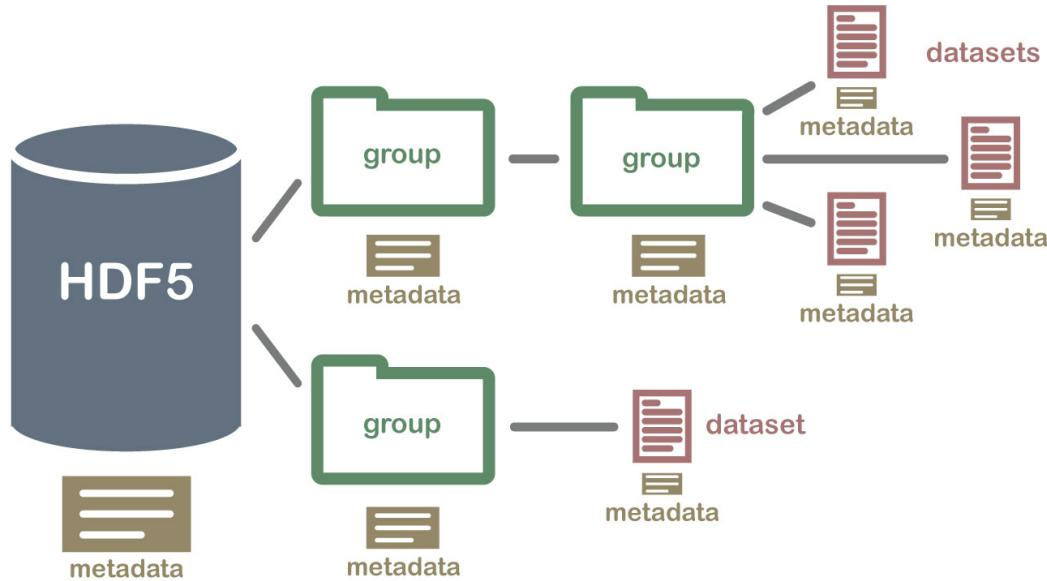
Beamformed LOFAR data uses this structure, where the formatting of the HDF5 file name in sub-array pointing, beam, and Stokes parameter, is represented in the file.
