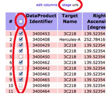
The LOFAR Archive stores data on magnetic tape. This means, that it cannot be downloaded right away, but has to be copied from tape to disk first. This process is called 'staging'.
