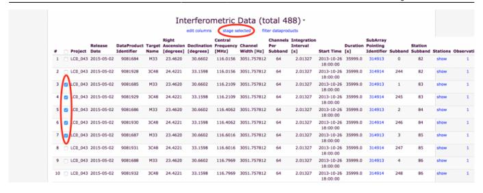
The LOFAR Archive stores data on magnetic tape. This means that it cannot be downloaded right away, but has to be copied from tape to disk first. This process is called 'staging'.
