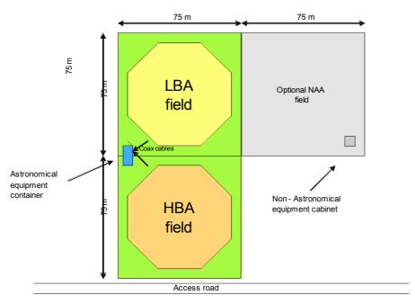
Figure 2-2 Remote station layout example 2
