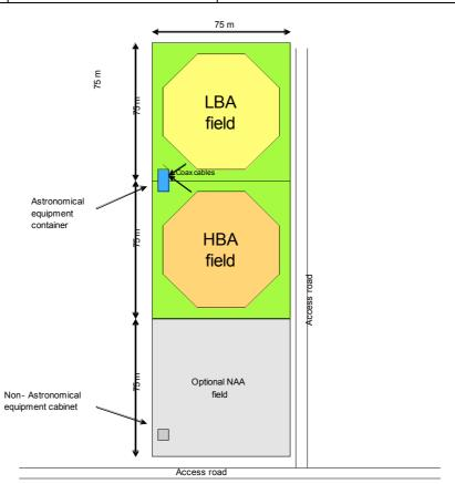
Figure 2-1 Remote station layout example 1
