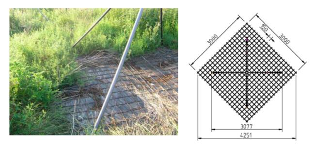
Figure 5-3: Ground plane with foil. Left: photo. Right: specifications.
