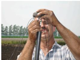
The antenna is connected with the two coax cables. There is a hole in the antenna such that the tube perfectly fits in the potted LBA.
