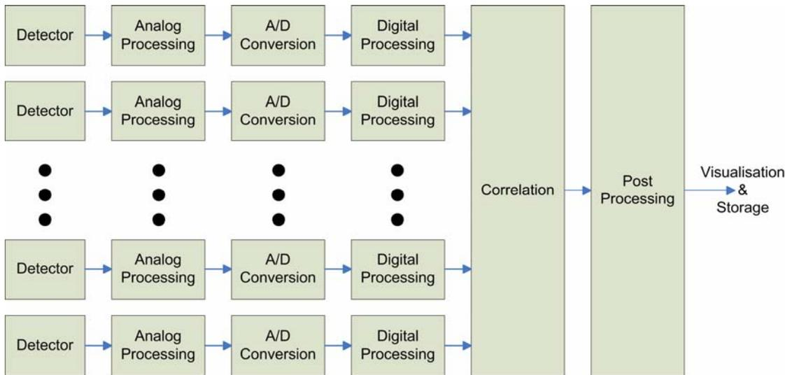
**Figure 3** General datapath of an aperture synthesis array
