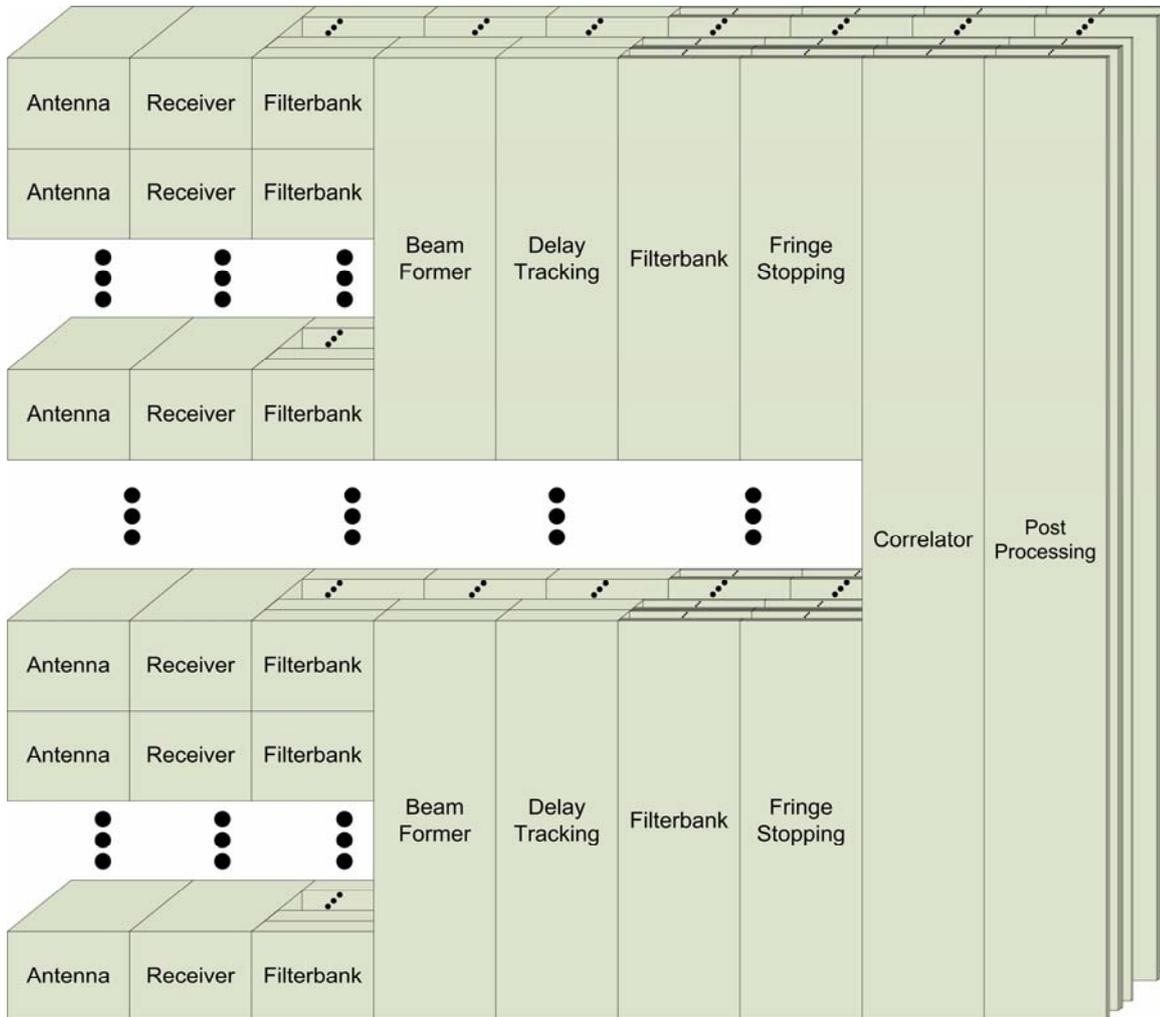
**Figure 8** Detailed LOFAR signal data path. The third dimension represents the frequency domain. For example the first filterbank splits up the digital signal into subbands, while the second filterbank splits those subbands further up into channels.
