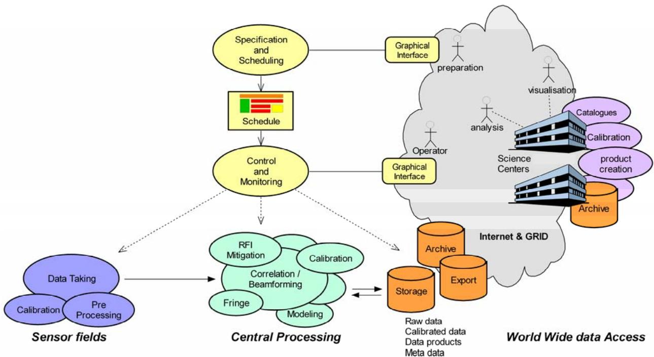
**Figure 16** Operational view on LOFAR. Shown is how the processing tasks at the bottom left of the figure are controlled through Specification, Scheduling, Control and Monitoring software. This management software is operated by the observatory staff and by the Science Centres when applicable. Detailed post-processing tailored to specific science needs may be done at the Science Centres.
