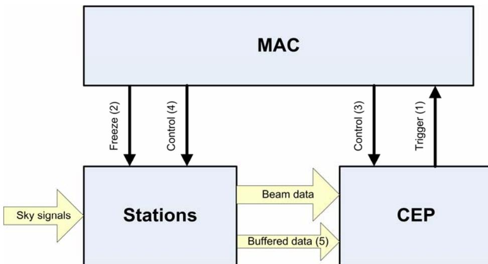
**Figure 18** HECR trigger scenario at system level (only the relevant signals are shown)
