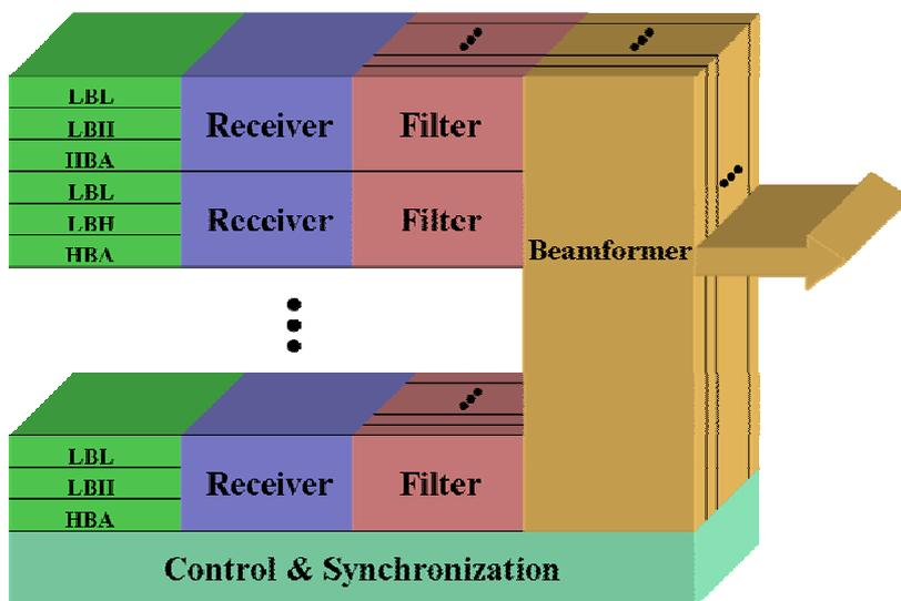
**Figure 9** Station architecture block diagram. The design covers three antenna systems which are connected to the receiver unit where analog filters dedicated for each antenna, can be selected. After digitisation, the antenna signals are filtered. Further beamforming is implemented per subband as indicated by the third dimension.
