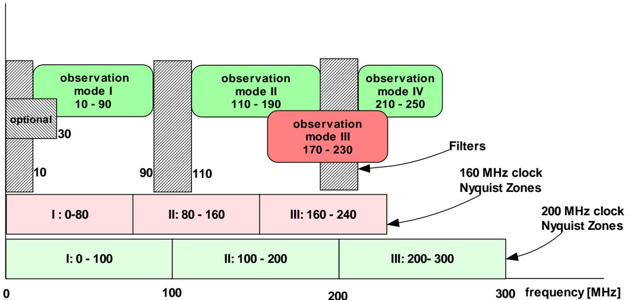
**Figure 10** Selection of Nyquist zones is used to select the observed band in the station.
