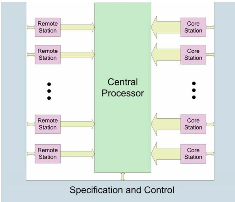
**Figure 4** LOFAR concept composed of remote stations, core stations, central processor, a specification and control layer and the transport between all. The width of the arrows identifies to some extent the amount of data transported.
