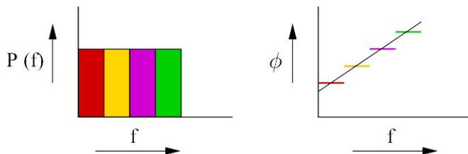
**Figure 7** Illustration of 4 subbands and the error which is introduced by approximating the time delays by phase shifts per subband (the black line on the right hand side is the ideal phase)
