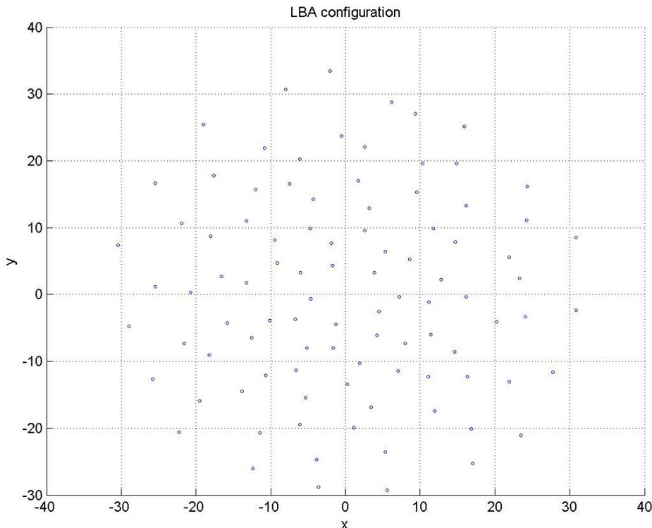
**Figure 15** LBA configuration of one of the stations currently in the field (axes scales are in meters)
