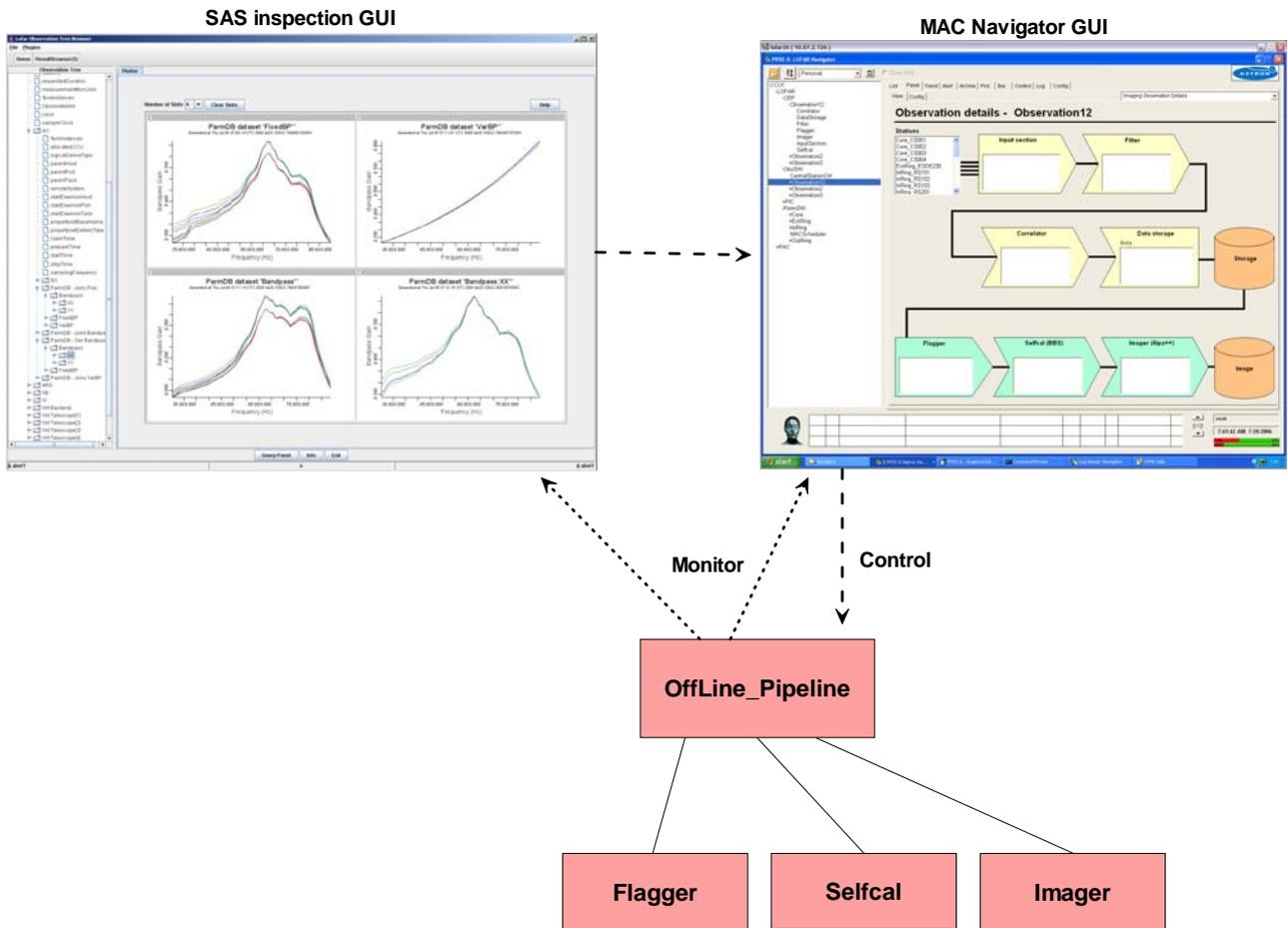
**Figure 17** Illustration of interactive control over a processing pipeline. In this example an imaging pipeline is inspected and controlled interactively by the SAS and MAC GUIs. As described in the text, this interactive usage is possible in the context of the full MAC control system.
