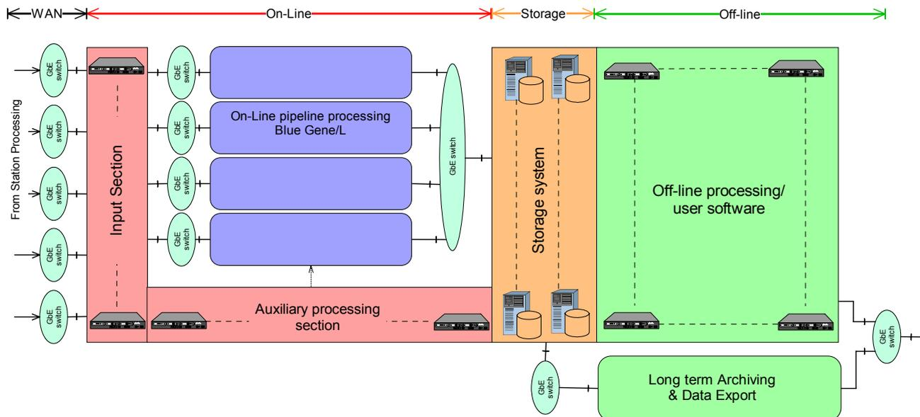
**Figure 11** Central Processor Facility hardware architecture overview. Four Blue Gene/L racks are embedded in a hybrid cluster computer. The sizes of the various parts of the cluster are scalable.
