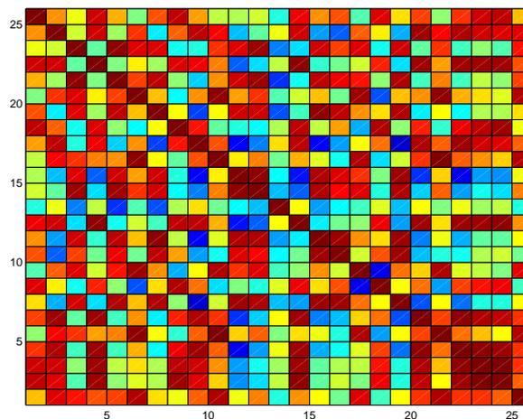
Figure 8: ITS Antenna Correlation matrix (ordered by antenna number)
