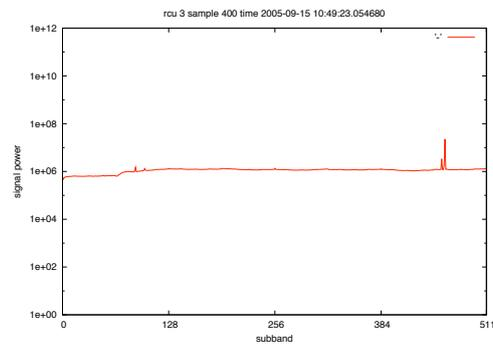
Figure 6: Typical 'Low Signal' subband statistics
