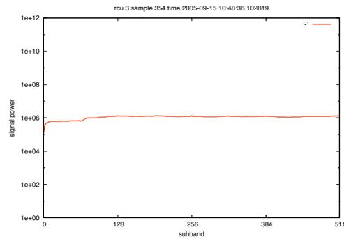
Figure 5: Typical 'No Signal' subband statistics
