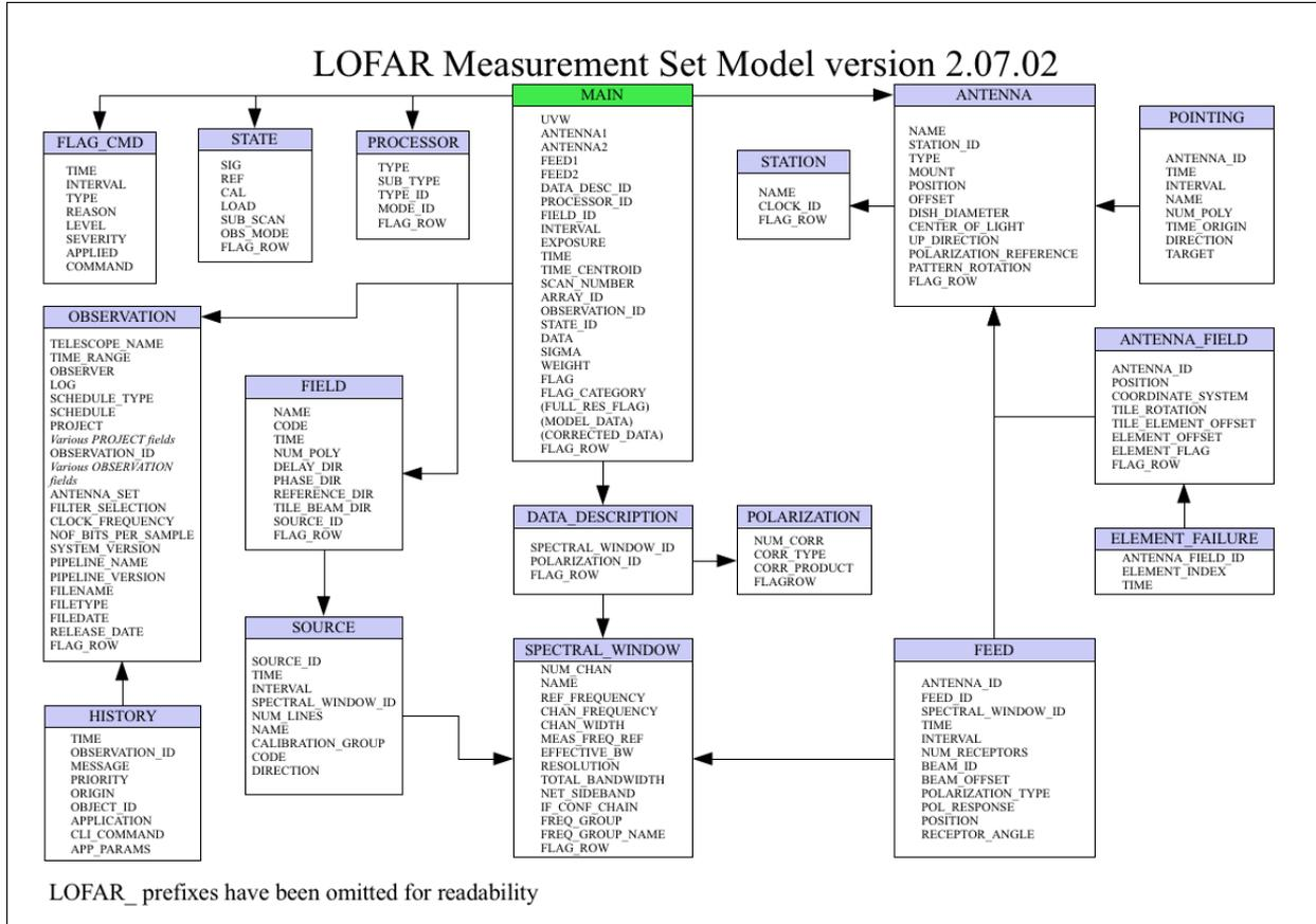
Figure 1: Schema of the LOFAR Measurement Set
