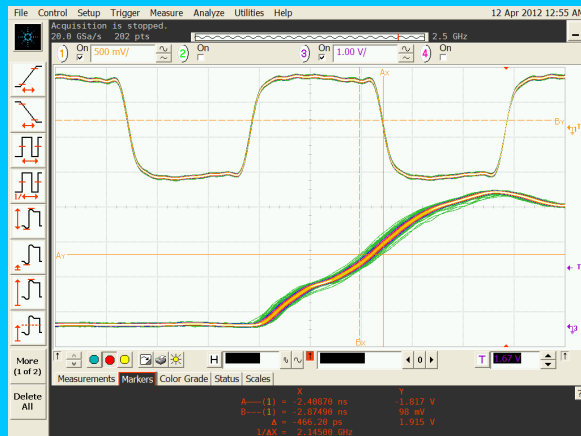
Figure 27 Effect of FS725 temperature sweep (10°C till 40°C) with SyncOptics
