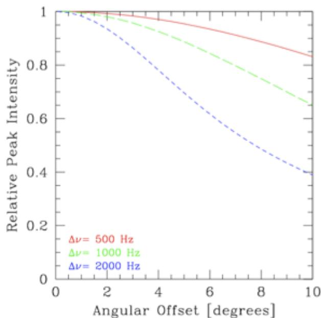
Figure 5: Demonstration of the effect of bandwidth and time average smearing on the relative peak intensity. The relative peak intensity is shown as a function of angular offset from the phase centre. For these 50 MHz observations using 0.25s integration time, curves are shown for three different channel bandwidths. Uniform weighting is used.
