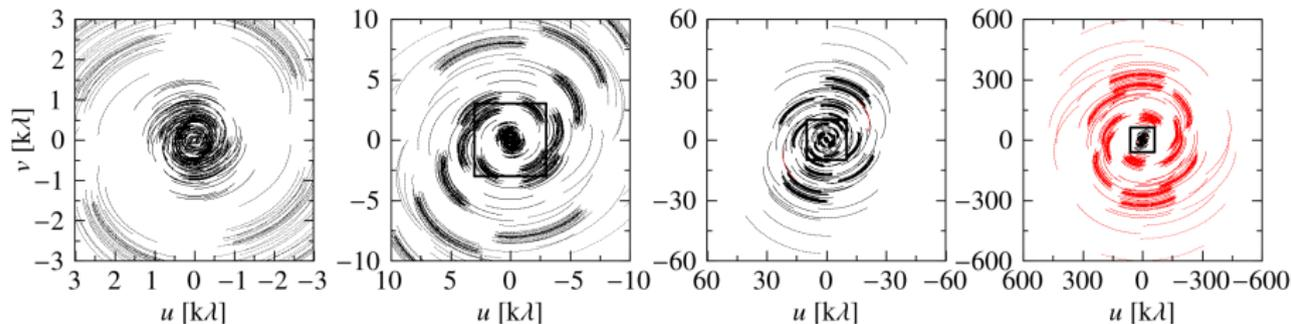
**Figure :**  $uv$  coverage for a typical 4-hr observation of a source at declination  $+48^\circ$  with a single subband centred at 140 MHz. Only one visibility every 160 seconds is shown. The rectangles in the last three panels show the area covered by the previous panel. Visibilities corresponding to baselines with international stations are plotted in red.
