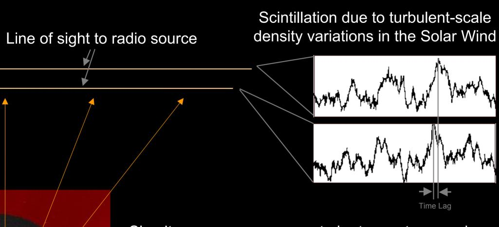
Simultaneous measurements by two antennas show similar patterns of scintillation.
