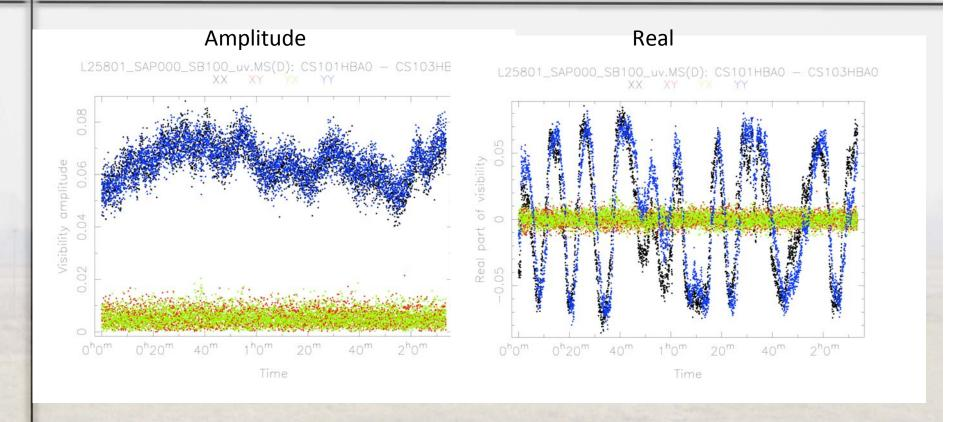
In dt=2s and df = 16ch (48.6 kHz) we find a S/N =14.3 For a flux density of  $S = 83 \text{ Jy} \rightarrow \text{noise} \sim 5.8 \text{ Jy}$
