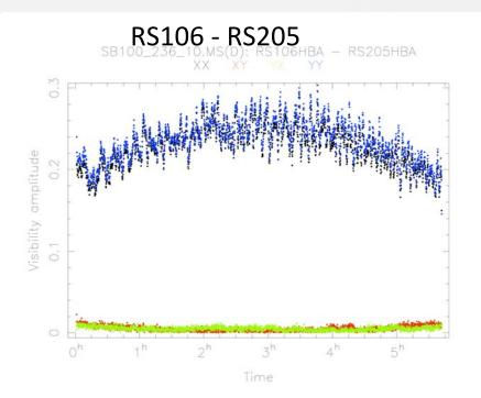
The XX and YY signals reflect the  $\sim$  83 Jy source 3C196 and its mucht fainter companion. The XY , YX signals still have a variable leakage component (and possibly some DFR).
