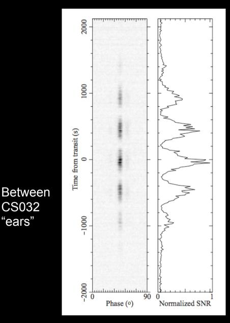
Try a drift-scan of PSR B0329+54 to map beam and check for coherency.
