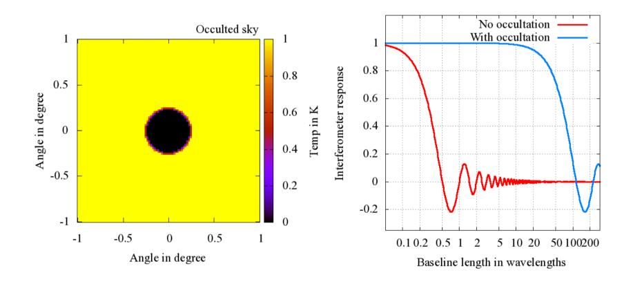
But .... interferometers measure the brightness difference between the occulting object  $T_{_{\rm M}}$  and the background  $T_{_{\rm B}}$
