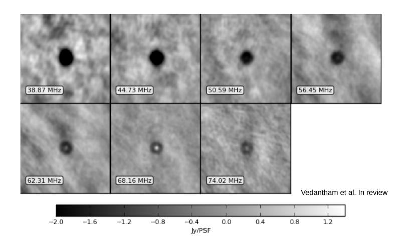
Reflected RFI (Earthshine) images to the center of the lunar disc, due to specular nature of reflection
