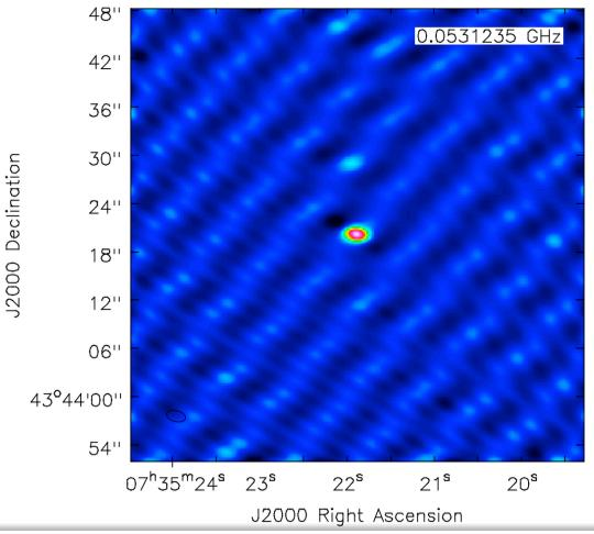
Point source model in, no selfcal, single timeindependent amplitude correction for the international stations: still recovers double-lobed structure!
