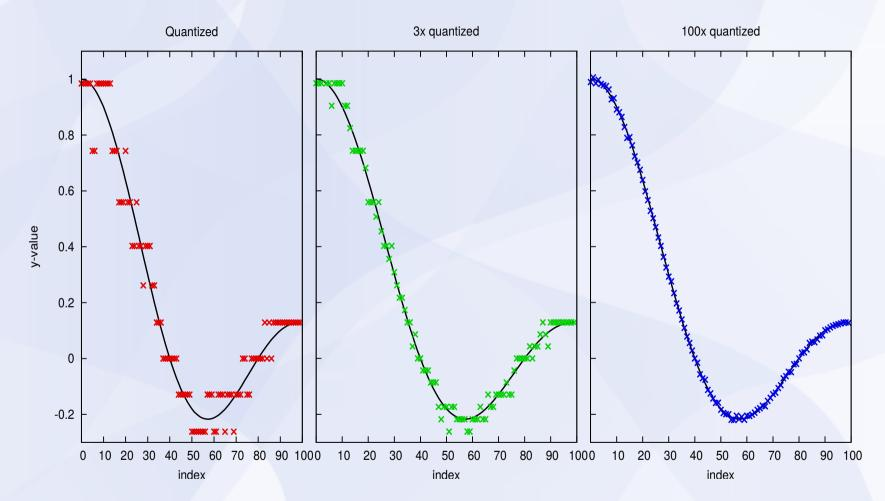
Fig. : A quantization example using the Gaussian-optimized least-squares quantization scheme with dithering to quantize a sinc function. 4-bit quantization and a single scaling factor were used. Left plot: result of encoding and decoding. Because the quantization is optimized for Gaussian distributed values, the quantization steps are smaller near zero. Central and right plot: average of 3 and 100 times encoding and decoding respectively.
