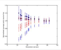
Selfcalibrated in red and GSM calibrated in blue. o's are the integrated flux and +'s are the peak flux of isolated FIRST point sources.
