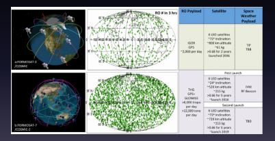
Comparison between (a) FORMOSAT-3/COSMIC and (b) FORMOSAT-7/COSMIC-2 in (left) constellation, (middle) RO events during 3 h, and (right) key parameters. Credits Yue, X. et al.
