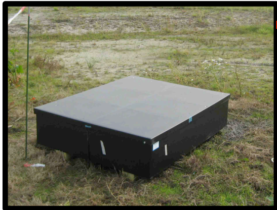
LORA LOFAR Radboud Array scintillator detectors
