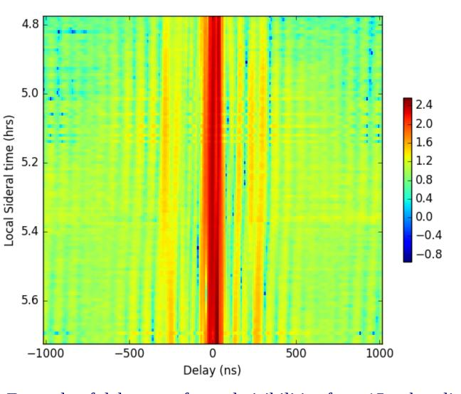
Example of delay transformed visibilities for a 15 m baseline integrated over 20 days
