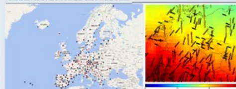
Fig. 6: EPN stations used in TEC (blue dots) and ROT (red dots) elaboration.
