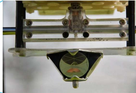
The UAV position is determined by the MTS at about 5 Hz rate
