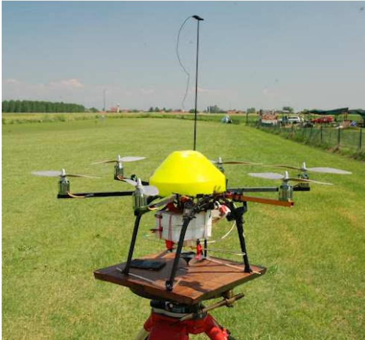
**Our UAV is a hexacopter (Mikrokopter KGPS v1.0) is a custom product based on commercial components, with engines and some electronic parts modified.**
