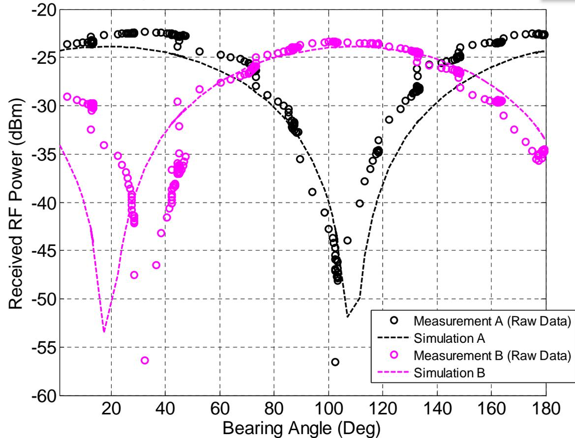
At this frequency the two antenna polarization planes are not perfectly aligned
