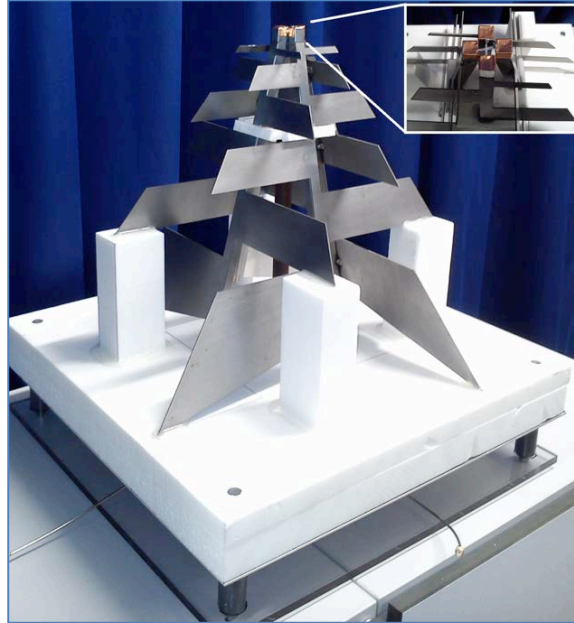
Second prototype Single ended feed
