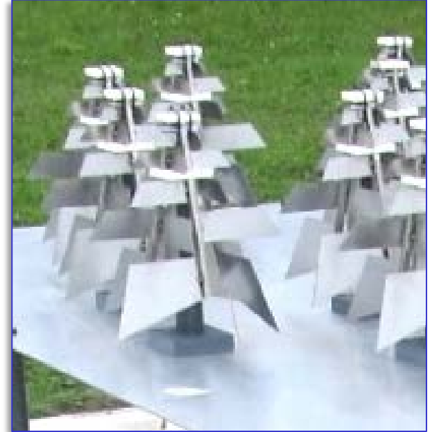
Third prototype Single ended feed
