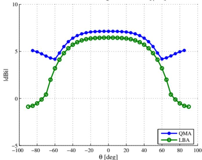
Quad-mode antenna achieves a gain variation below 3dB over the scan range from  $-90^\circ$  to  $90^\circ$
