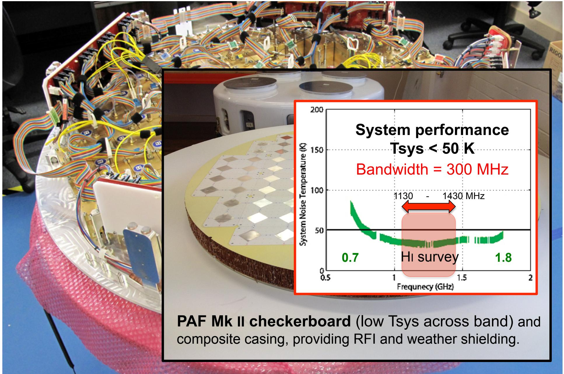
**PAF Mk II checkerboard** (low  $T_{sys}$  across band) and composite casing, providing RFI and weather shielding.
