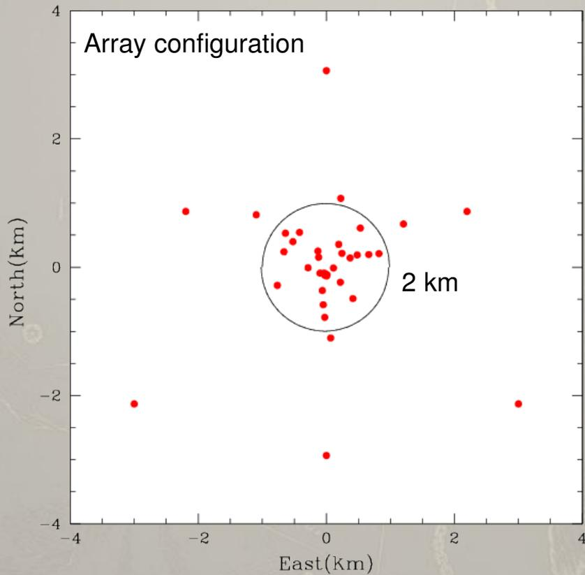
“The initial array configuration for ASKAP” (Gupta, Johnston, Feain, and Cornwell 2008)
